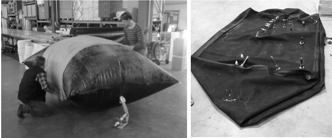
Fig. 2: Leak tightness test of a flexible rubber tank (left), tank with a storage volume of 5 m 3 and in-/outlets (right)
